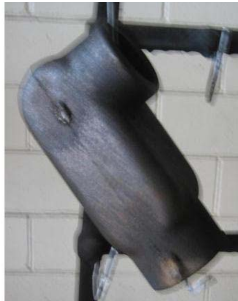
Alternative Hanging Practice. Water flows completely out of the part.
